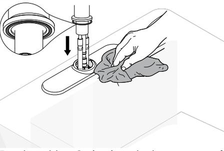
Put the rubber O-ring into the bottom gap of faucets then Insert faucet into faucet hole.
