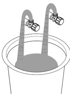
Shut off water suppliers. Remove the old faucet, clean the mounting surface.
