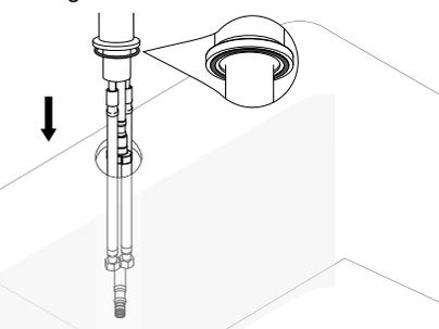
Put the rubber O-ring into the bottom gap of faucets then Insert faucet into faucet hole.
