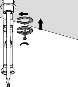
From underneath the countertop, Slide rubber washer, metal washer and mounting bracket onto the thread shank.
