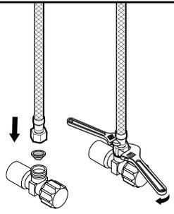
Connect and tighten the supply hoses by using two adjustable wrenches (avoid twisting or kinking).
