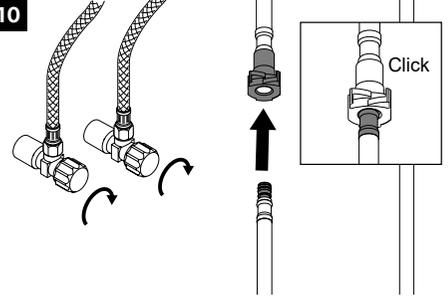
Shut off water suppliers. Push the handspray hose(7) into the quick connector(10) until you hear a click sound. Make sure it's secured.
