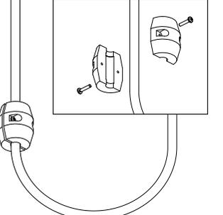
Install the hose weight on the outlet side of the hose, near the loop.
