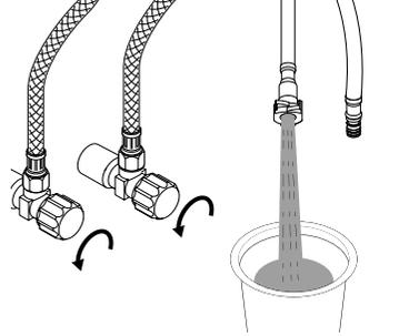
Turn on water suppliers. Place a bucket below outlet tube, slowly open and close the supply angle valves, **This will prevent debris from being lodged in the hose and sprayer.**
