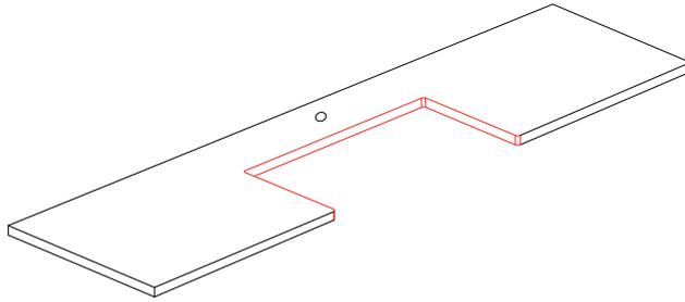
Measure the size of the sink, including the front apron. Cut the countertop to allow the sink slide in.
