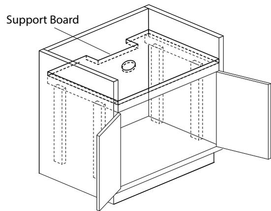
This step to ensure the bottom of the sink has enough support
