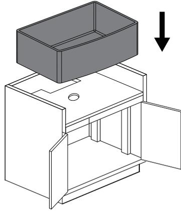
Using two people, carefully place the sink in place. Verify that the sink can fit in the cabinet opening and rest properly on the supporting system. Make a small adjustment to fit as necessary. Verify the overall appearance and check for levelness to ensure correct drainage.
