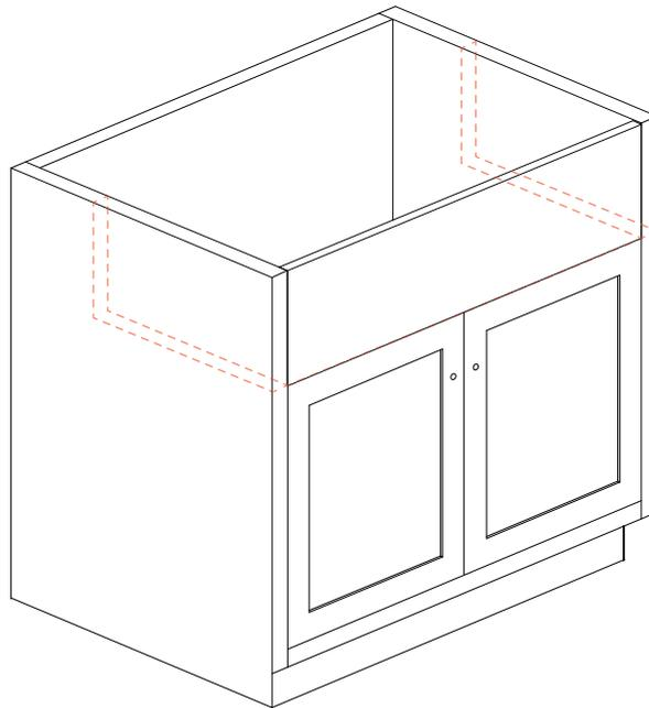
Measure the size of the sink, including the front apron. Cut the face of the cabinet to allow the sink slide in. Use painter's tape for marking and cutting purpose to protect the cabinet and sink from damage. KIBI recommends to install the sink under the counter, if you want to install flush or semi-recessed, be sure to adjust the height and length of the cabinet cut.
