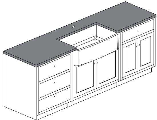
After cleaning, apply a bead of silicone sealant between the top flange (or lip) of the sink and the countertop to create a watertight seal. Clean excess silicone immediately. Verify the overall appearance and check for levelness to ensure correct drainage. Carefully place the countertop and verify that it is level.
