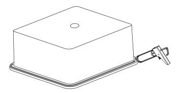
Turn the sink over and apply a generous bead of silicone sealant along the bottom of the sink rim.
