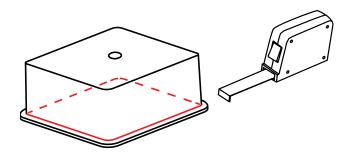
Measure the width of the underside of the sink rim.
