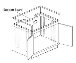
This step to ensure the bottom of the sink has enough support
