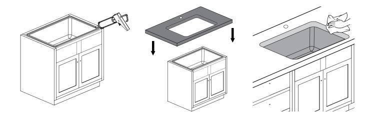
After cleaning, apply a bead of silicone sealant between the top flange (or lip) of the sink and the countertop to create a watertight seal. Clean excess silicone immediately. Verify the overall appearance and check for levelness to ensure correct drainage. Carefully place the countertop and verify that it is level.
