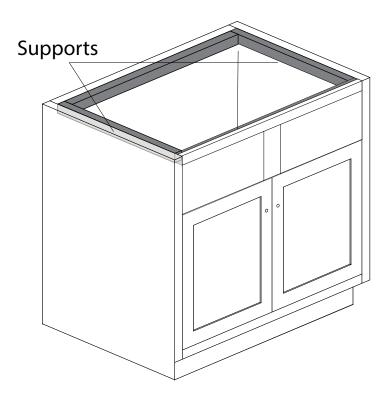
Construct a wooden frame to support the sink. Measure your sink to determine the dimensions.
