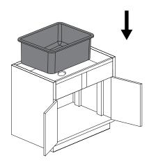
Using two people, carefully place the sink in place. Verify that the sink can fit in the cabinet opening and rest properly on the supporting system. Make a small adjustment to fit as necessary. Verify the overall appearance and check for levelness to ensure correct drainage.
