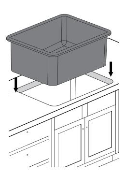
Insert the sink into the opening, check the alignment of the sink to the cutout in the countertop and press firmly.
