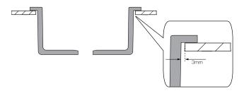
Subtract 3 mm from the width of the underside of the sink rim, and then subtract this amount from the perimeter you have drawn.
