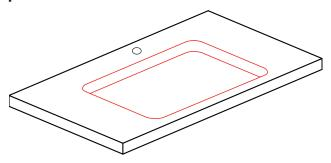
Measure the size of the sink. Cut the countertop to allow the sink slide in.
