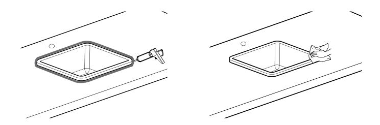
After cleaning, apply a bead of silicone sealant between the top flange (or lip) of the sink and the countertop to create a watertight seal. Clean excess silicone immediately. Verify the overall appearance and check for levelness to ensure correct drainage. Carefully place the countertop and verify that it is level.
