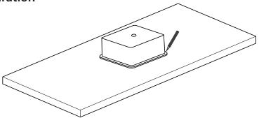
Place the Sink in the required position and use it as a template to draw around its perimeter.
