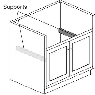
Build structural supports on the inside frame of the sink base cabinet. The structural supports must support the weight of the sink and any attachments such as garbage disposals.
