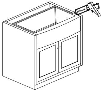
Set the sink on top of the cabinet or into the cabinet front cutout. Apply sealant if necessary as a gasket between the sink and cabinet.
