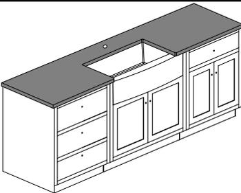
Carefully clean bottom of countertop and top edge of sink with denatured alcohol. Apply a bead of silicone adhesive (not supplied) around the top edge of the sink. Place countertop onto the sink.
