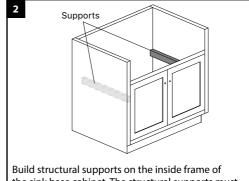
build structural supports on the inside frame of the sink base cabinet. The structural supports must support the weight of the sink and any attachments such as garbage disposals.
