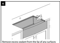
Remove excess sealant from the lip of any surfaces with a cleaner recommended by manufacture of adhesive sealant.
