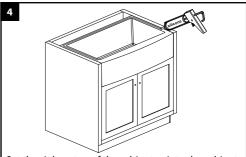
Set the sink on top of the cabinet or into the cabinet front cutout. Apply sealant if necessary as a gasket between the sink and cabinet.
