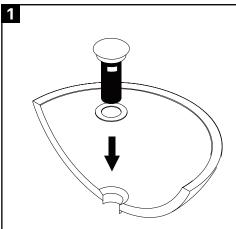
Remove all components from drain piece including: thin and thick silicone washer, hard washer, drain nut and tail piece.
