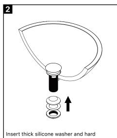
Insert thick silicone washer and hard washer over the exposed mail threaded area and screw drain nut onto drain. Do not overtighten.
