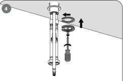
From underneath the countertop, Slide rubber washer, metal washer and mounting bracket onto the thread shank.
