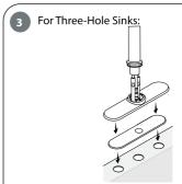
Put the rubber O-ring into the bottom gap of faucets then Insert faucet into faucet hole.
