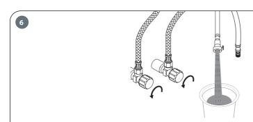
Turn on water suppliers. Place a bucket below outlet tube, slowly open and close the supply angle valves, **This will prevent debris from being lodged in the hose and sprayer.**
