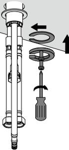
From underneath the countertop, Slide rubber washer, metal washer and mounting bracket onto the thread shank.
