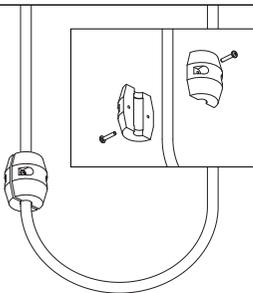
Install the hose weight on the outlet side of the hose, suggested installation position is marked on the hose.
