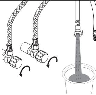
Turn on water suppliers. Place a bucket below outlet tube, slowly open and close the supply angle valves, **This will prevent debris from being lodged in the hose and sprayer.**
