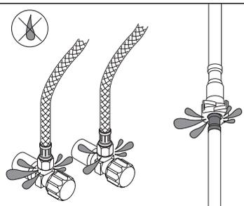
Turn on the water suppliers, Shut off the faucet and check for leaks.
