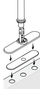
Put the rubber O-ring into the bottom gap of faucets then Insert faucet into faucet hole.
