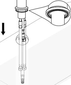
Put the rubber O-ring into the bottom gap of faucets then Insert faucet into faucet hole.
