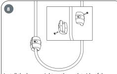
Install the hose weight on the outlet side of the hose, suggested installation postion is marked on the hose.
