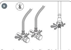
Turn on the water suppliers, Shut off the faucet and check for leaks.
