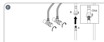
Shut off water suppliers. Push the handspray hose(A) into the quick connector(B) until you hear a click sound. Make sure it's secured.
