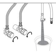
Turn on water suppliers. Place a bucket below outlet tube, slowly open and close the supply angle valves, **This will prevent debris from being lodged in the hose and sprayer.**
