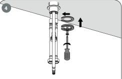
From underneath the countertop, Slide rubber washer, metal washer and mounting bracket onto the thread shank.
